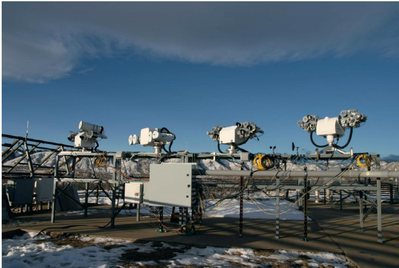
FIG. 1. The 33 pyrheliometers mounted on four trackers for the 10-month comparison. The four windowed cavity radiometers are on the second tracker from the left. (Credit: Stephen Wilcox, NREL.)
